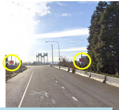
Relocated Approximately 150 ft further south to give drivers more time to see the blinking LED warning signs
