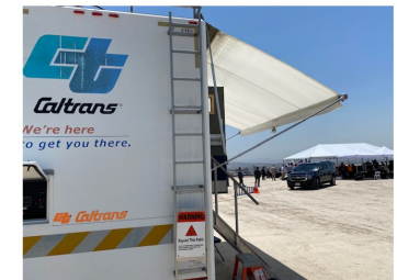
Place safety sign on ladder to prevent accidental exposure to microwaves.
