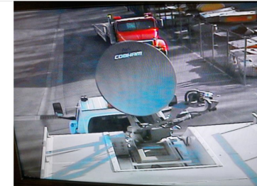
As dish deploys if it looks like it will hit trailer TURN OFF controller.
