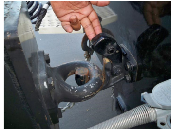
Next is to level trailer. Release pintail hook – remove key.
